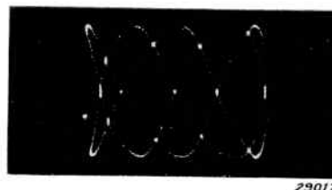
Fig. 7. Lissajous figure which occurs when the frequencies of the vertical and horizontal deflecting voltages are in the ratio 5/2 .
