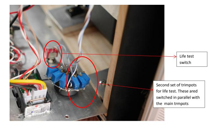
For the life test (reduce filament voltage by 10%) there is another set of trimpots that the rotary switch connects in parallel with the first set of trimpots on the switch. This second set of trimpots in parallel reduces the overall resistance which reduces the output voltage from the board.
