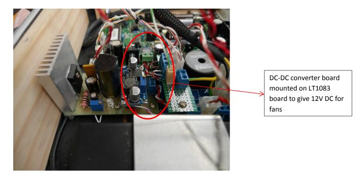
I used the standard heatsink in the kit for the LT1083. This heatsink is quite small but is ok for up to about 1.6A heater supply for KT88 valves.
