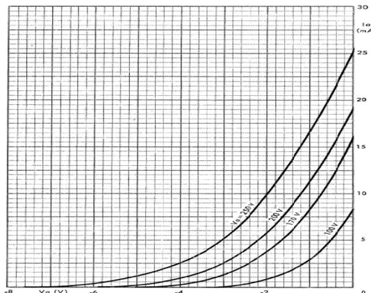
**JAN6922**, is a military spec 6DJ8 / ECC88 twin triode tube developed as RF low noise.
