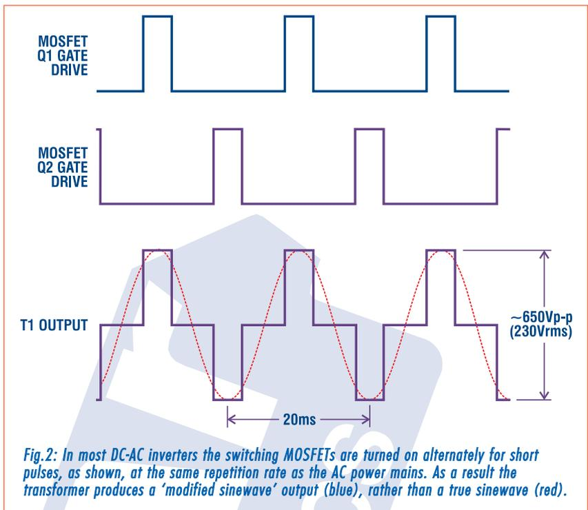
**Fig.2:** In most DC-AC inverters the switching MOSFETs are turned on alternately for short pulses, as shown, at the same repetition rate as the AC power mains. As a result the transformer produces a 'modified sinewave' output (blue), rather than a true sinewave (red).
