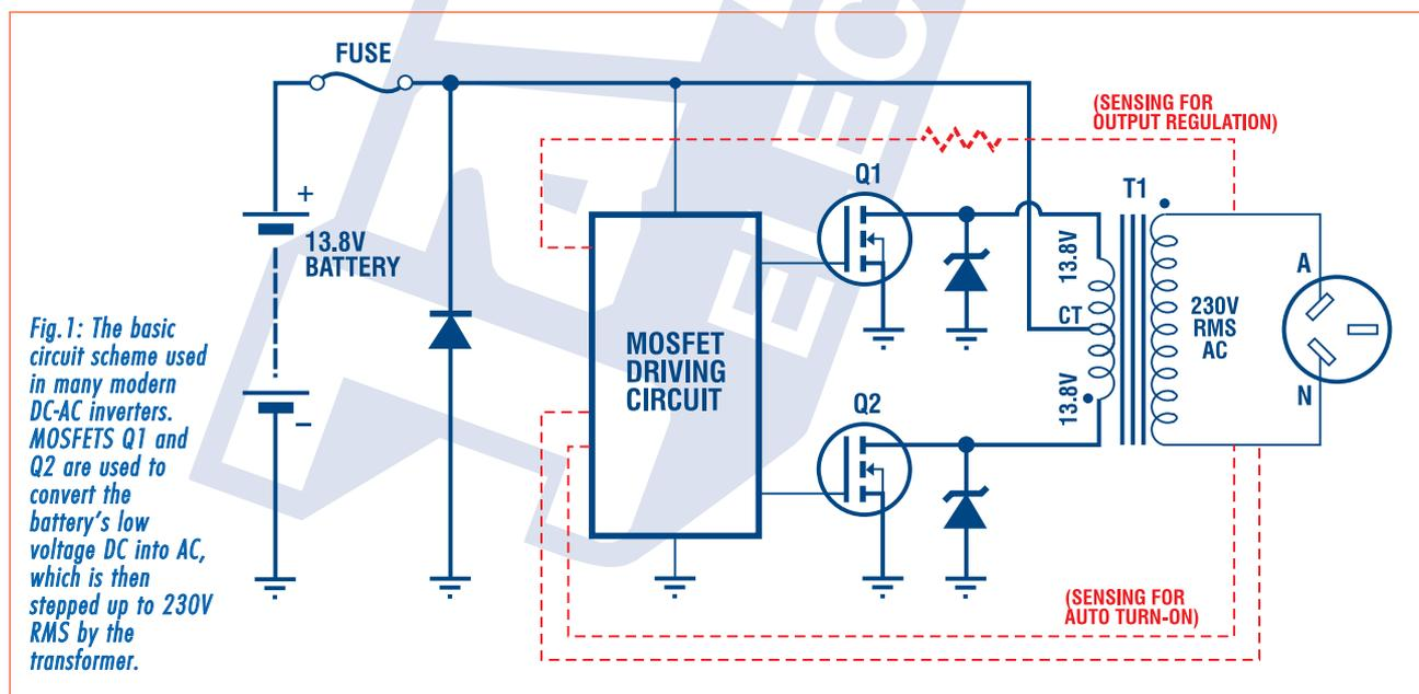
approach does have limitations, mainly because it can generally only increase the pulse width to a certain point. (In the extreme, the output becomes a square wave.) This may not be sufficient to allow the inverter to deliver enough RMS output voltage in short-term overload or 'surge' conditions.
